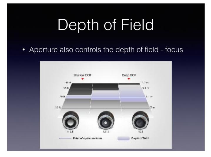
Depth of field: the amount of the image that is in focus. A band of data across the width of the image. Closer or further objects out of focus. The closer the object that is focused on, the smaller the depth of field.
